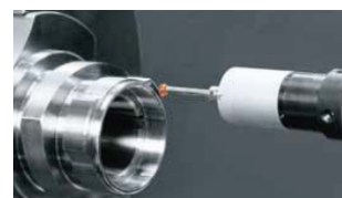
工件自动测量 Automatic measurement of workpieces
